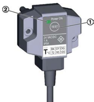
Fig. 39: Mecanism de declanșare termoelectric BAT
