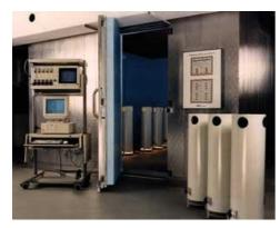
This facility is used for the standardised identification of the cooling capacity of passive water cooling systems according to standards DIN EN 14240, 14518 and 15116. This is where new developments are advanced, catalogue data determined and measurements are taken as proof of performance for major projects according to
