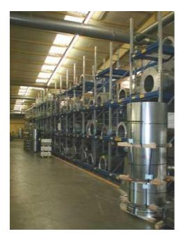
We are mainly working with flat products such as sheet metal and tapes. Most of the material has been galvanised DX 51 D+Z with a pressure by load of approx. 150 gramme per  $m^2$ .
